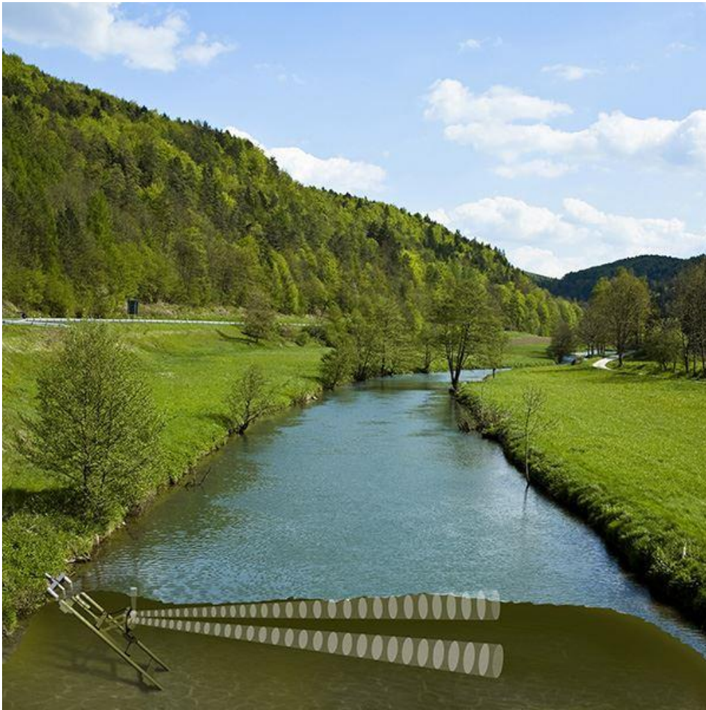
Figure C.6. Conceptual diagram illustrating the acoustic Doppler “ladder” array configuration used for velocity profiling and discharge estimation. (Generic reference image; not from Niqliq site) (Source: Xylem, 2025)
