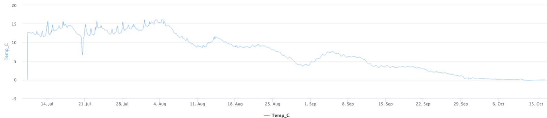
Figure A.1. Water Temperature (°C) — Open-Water Cooling Sequence, Niqliq Channel, July–October 2025. (Source: Xylem Hydrosphere Network, 2025 — Niqliq Channel Station)
