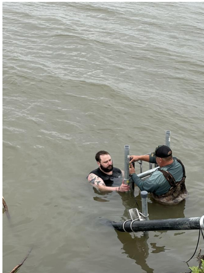
Figure C.9. Xylem and NVN DNR team securing in-water sensor assembly for the YSI EXO2 unit. (NASA, NVN DNR, 2025)
