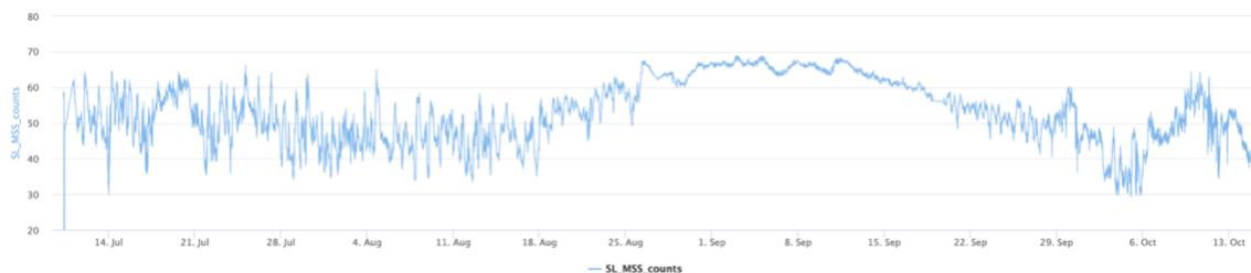
Figure 7.4. Signal Strength (MSS counts) — SonTek SL Acoustic Doppler Current Profiler, July–October 2025. Signal returns remained within the 45–70 count range throughout deployment, confirming consistent acoustic transmission quality despite high turbidity during late-August flood events.
